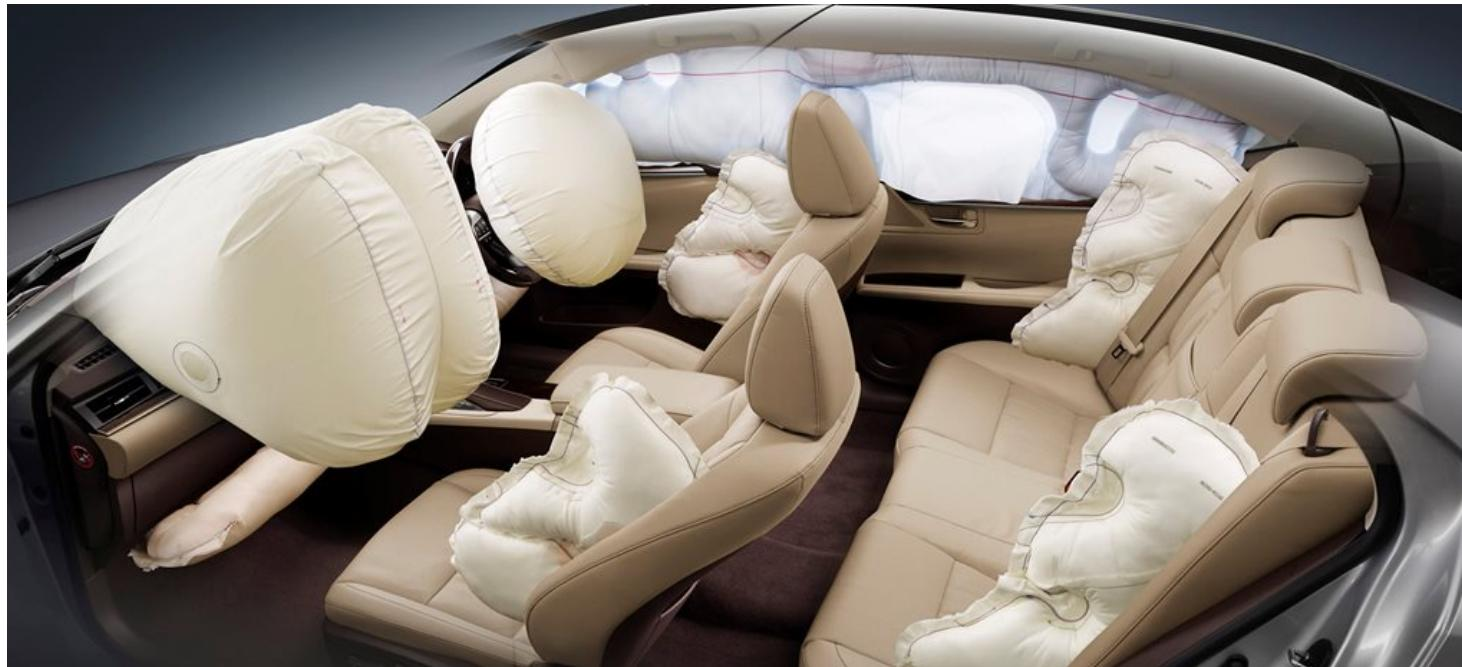
The airbag does not reduce the likelihood of a car accident occurring, but if an accident happens, it helps reduce the impact on the passenger.
