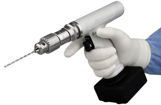
Medical drills are equipped with a speed controller that automatically cuts the current to the motor if the rotational speed exceeds the predefined safety limit, preventing potential tissue damage and ensuring precise surgical performance.
